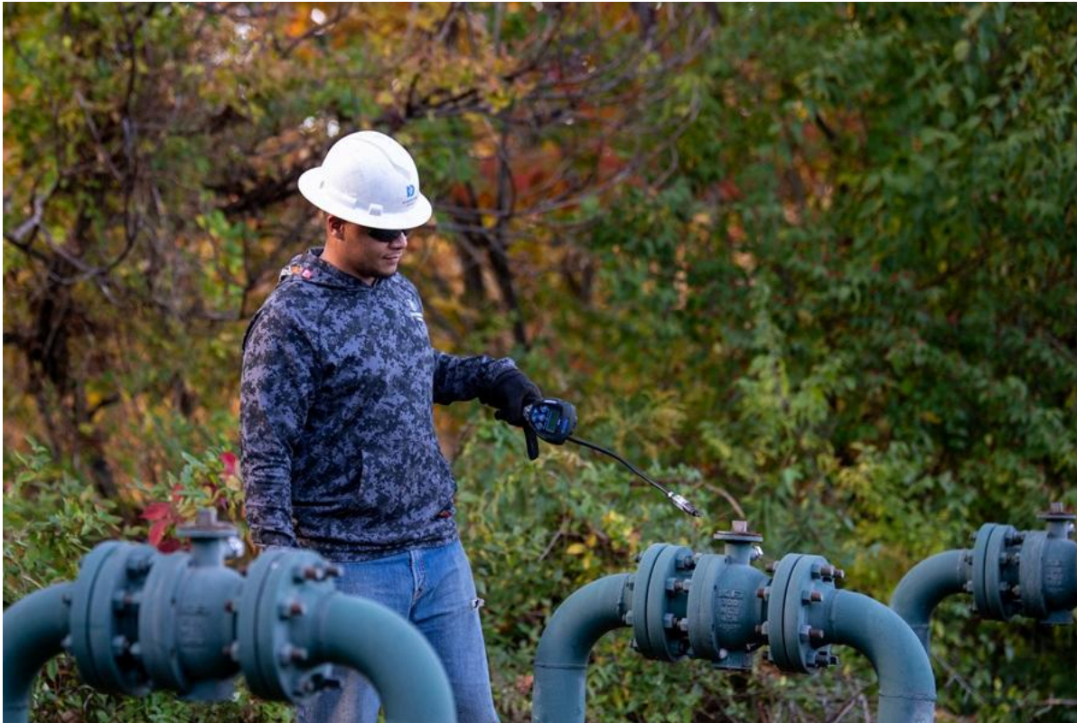
Diversified's suite of handheld emissions technologies includes the Teledyne FLIR GT-44. Well tenders survey wells across the company's operating areas. (Source: Diversified Energy)
