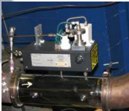
DSHF sampling assy installed on engine dyno exhaust. No heated lines required
