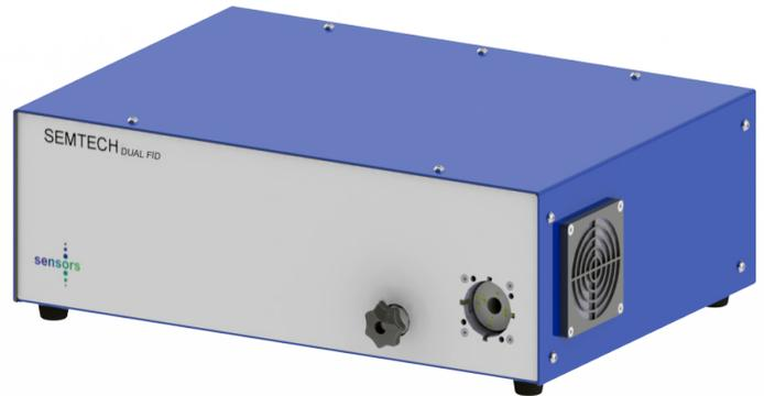
The system is designed to minimize the loss of hydrocarbons prior to analysis by maintaining the required temperature through the use of a heated filter, heated sample line and stainless steel fittings, all of which have low hydrocarbon adsorption characteristics. User-selectable measurement ranges ensure accuracy for a wide variety of test applications.
