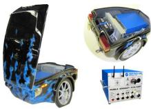
Sensors' Emissions Trailer and **SEMTECH-DS Gaseous Emissions Analyzer**
